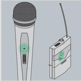
Green: battery is OK and transmitter is operational; Red: replace battery soon; Does not light up: replace battery now
