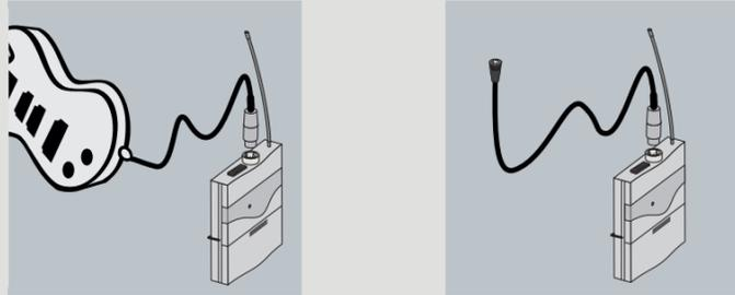
Connect instrument or microphone to the mini-XLR jack of the pocket transmitter.
