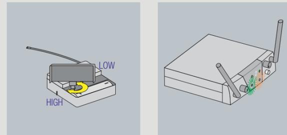
Adjust the input sensitivity on the PT40 pocket transmitter using the screwdriver included in the battery compartment cover:
