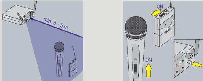
Observe minimum distance between transmitter and receiver.
