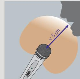
In the case of microphones with a cardioid polar pattern, most sound attenuation occurs at 180°. These microphones should therefore preferably be used where there is an interference noise source or a loudspeaker directly opposite the speaker. Holding the microphone less than 5 cm from your mouth will give your voice a voluminous and punchy quality.
