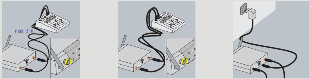
Connect receiver to a balanced **OR** unbalanced input!
